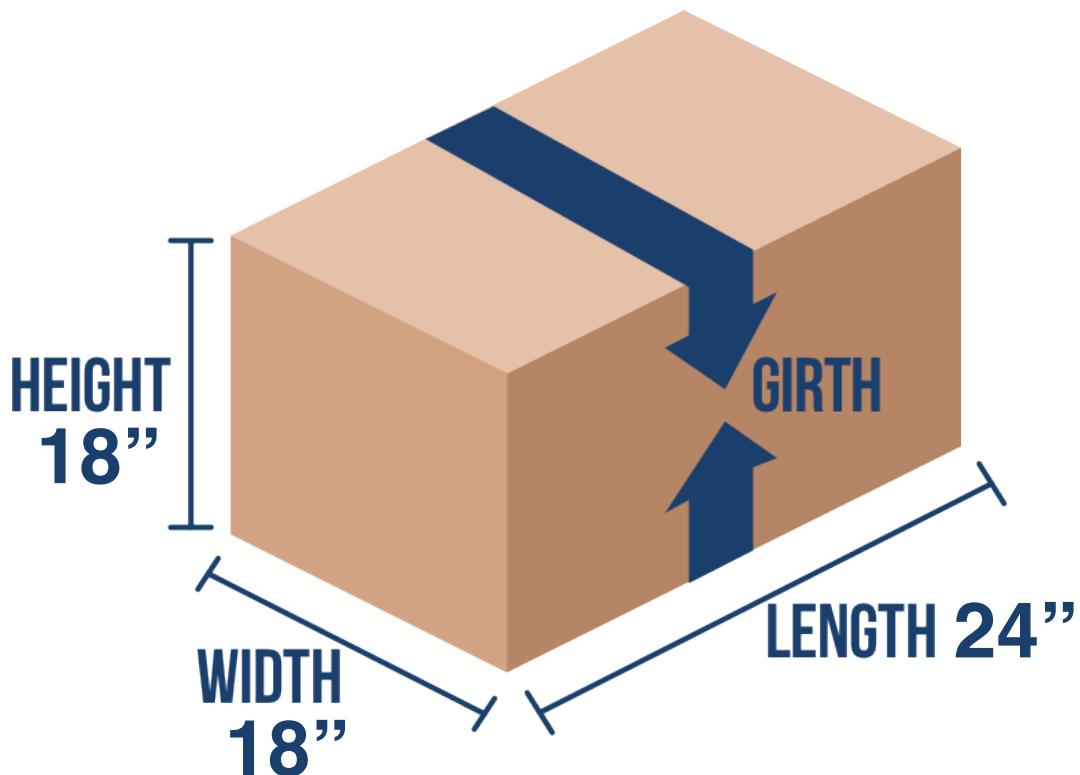
$2 \times \text{Height} + 2 \times \text{Width} + \text{Length} = \text{Girth}$
